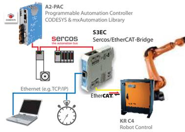
□ A2-PAC control with CODESYS and mxAutomation library communicating in real-time with a KUKA KR C4 robot control. (Source: KUKA Roboter GmbH)
