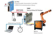
A2-PAC control with CODESYS and mxAutomation library communicating in real-time with a KUKA KR C4 robot control. (Source: KUKA Roboter GmbH)
